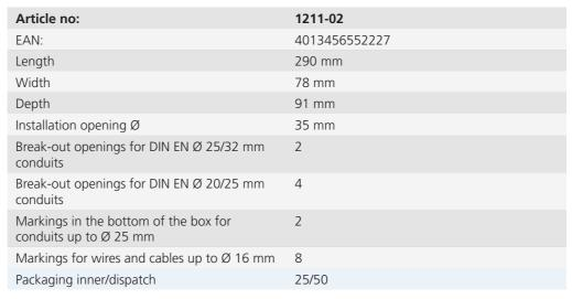
The new Prefix® concrete construction boxes, in addition to the proven product features such as lateral installation clamps for fastening to the reinforcement, mounting clips for pre-fixing the items and marked wave profile for an exact and secure fit, now also have innovative conduit entries, insertion options in the rear part of the box as well as separators that can be broken out at a later date for connecting devices in combinations.
