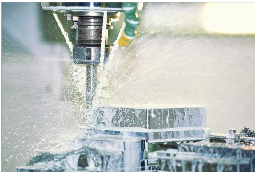
Fig. 5: 'Liquid cooling solutions' are suitable for the most demanding applications, such as milling machines with precision spindles, where an imprecise cooling temperature would have a negative effect on the machining tolerances of the workpiece.
