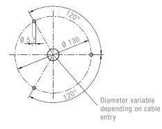
Two different drilling templates are available for fixing the light (direct mounting). M5x 8 threaded bushes are set into the base of the light for fixing according to drilling template 1. Drilling template 2 allows the light to be fixed using 4 through bolts or similar from above.
