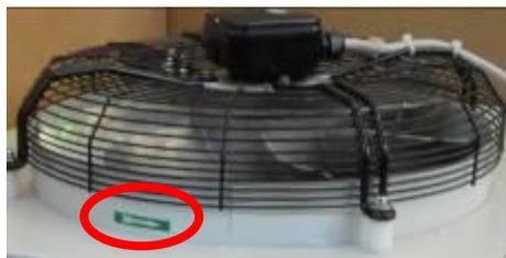
Picture 21 – Fan rotating direction
